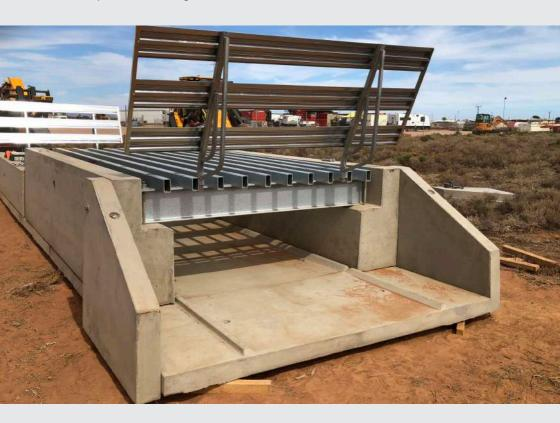
Our headwall's unique design help minimise erosion at the ends of the abutments. They are bolted to the end of the abutments and back filled with appropriate soil.
