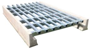
This grid is suitable as a front gate replacement or used between paddocks. It can be provided assembled due to its light weight. The steel is fully hot dipped galvanised and is easily removed for cleaning.
